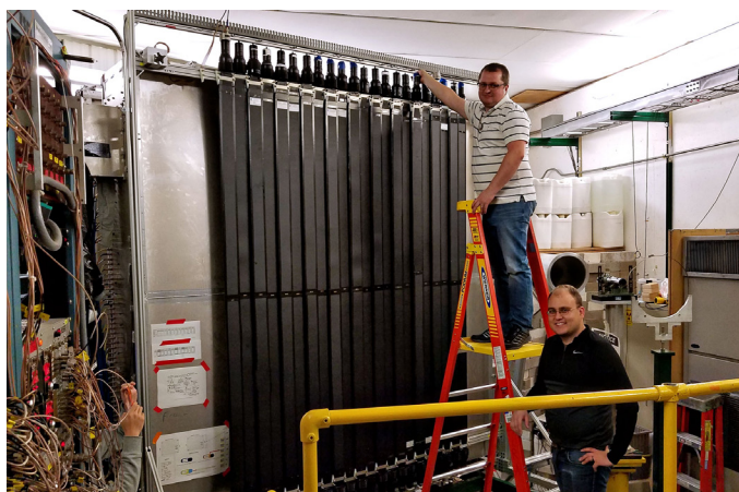
Zbigniew Chajeccki of Western Michigan University and Kyle Brown testing the particle veto wall (black vertical scintillation bars) installed in front of the Large Neutron Wall Array (only the Aluminum cover behind the veto bars is visible) in preparation for the commissioning of the veto wall.
