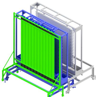
The 3D rendering of the arrangement of the veto wall (under construction) with the two neutron walls stacked behind. The horizontal Pyrex tubes containing the liquid scintillator NE213 are normally enclosed in an Aluminum casing for protection.
