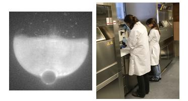
Left: A radiograph of the back-wall of the zirconium-88 collection container. The brighter areas indicate places where zirconium stuck to the material. The water-line is clearly visible across the top, and the drain-port is visible as the small circle in the bottom. Right: Hannah and Paige working in the newly finished radiochemistry laboratory.
